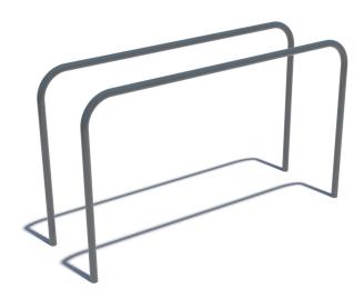
The construction consists of two curved bars that are placed parallel. The distance between the inside surface of the bars is 500 mm. The upper horizontal surface of the bars is 1650 mm long. Bars are symmetrically curved at the angle of 90 degrees and create the construction at the height of 1200 mm (1300 mm optional height is possible) from the foundations. Weight 52 kg.
