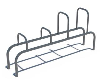
This is a metallic construction with base horizontal surface 2040 mm in length, 400 mm in width, and 500 mm in height. The construction has four semi-rings between which there is a distance of 500 mm, 394 mm and 500 mm accordingly. The height of the semi-rings: 250 mm and 250 mm, 500 mm and 500 mm. The construction consists of tubes with diameter from 34 mm to 50 mm. Weight 53 kg.
