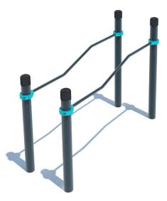
The complex consists of four vertical columns at the height of: 1500 mm -2 pieces, 1200 mm-2 pieces. Parallel bars are fixed to backup columns at the height 1000mm and 1300mm by means of collars. The distance between bars is 598 mm, total lenght 1790mm, bar diameter 42 mm. Construction is secured together with siluminium clamps
