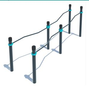
The complex consists of six vertical columns of different height, multi-width parallel bars 1790 mm in length and multi-level parallel bars 1790 mm in length. The distance between the multi-width parallel bars is 598 mm at the narrow end and 1198 mm at the wide end. Total width difference for the parallel bars is 600 mm. The difference between the lowest and highest point of the multi-level parallel bars is 300 mm. The structure is secured together with siluminium clamps. Weight - 137,00 kg.
